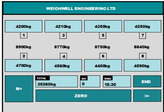
The weighing information can be reprinted many times. The USB function exports the weighing data into a csv file which can be used for more in-depth analysis.
