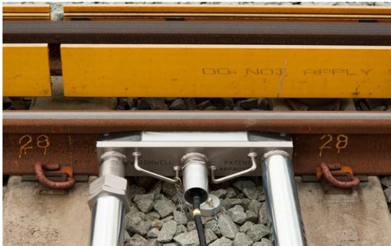
Our PTW allows for greater flexibility without the need to remove rail fastenings due to its length of only 500mm. This results in a more convenient installation without the need for expensive or time consuming civil works.
