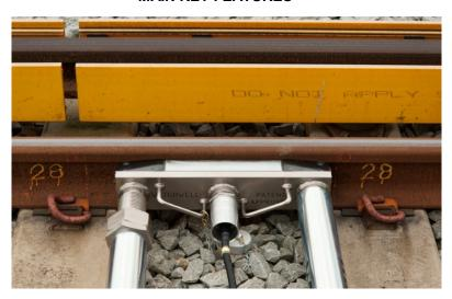
Our PTW allows for greater flexibility without the need to remove rail fastenings due to its length of only 500mm. This results in a more convenient installation and less 'flexing' of the system. The benefits of this are more accurate, repeatable and reliable weighing results.
