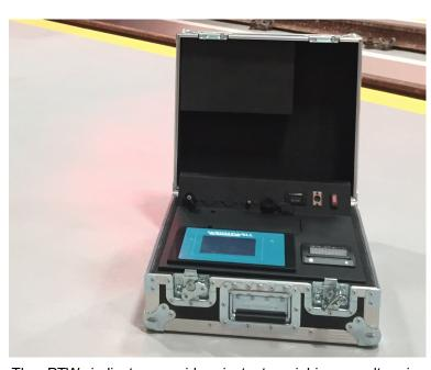
The PTW indicator provides instant weighing results via printout or CSV file. Operating via three main screens the robust and IP65 rated indicator provides easy to use functions and immediate weighing information.
