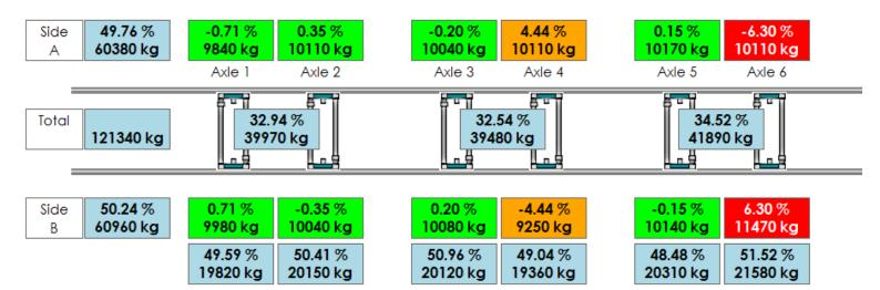
Our intuitive, multilingual ptwX software is designed and developed in-house and provides real time 'live' displays. Multiple customisations such as weighing units, wheel numbering and information on weight differentials (tolerances) are also available.
