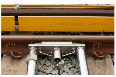
Our PTW allows for greater flexibility without the need to remove rail fastenings due to its length of only 500mm. This results in a more convenient installation without the need for expensive or time consuming civil works.
