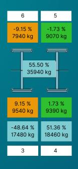
Designed for static weighing, this software captures the weights based upon your rolling stock configuration. The main features are adjustable tolerances for error conditions and wheel numbering specific to your rail vehicle.
