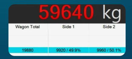
This in-motion weighing software, graphically highlights load imbalances as percentages or ratios. Key features include custom train setup (such as locomotive pushing or pulling) and raw data export.
